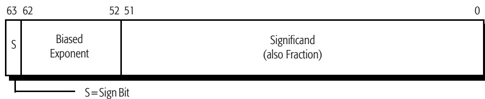
Figure 4-15. 128-Bit Media Floating-Point Data Types
